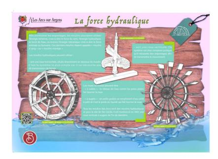
To drive the gears, the mills could use wind power, water power, or mechanical power (animal or human force). These mills were called "blood mills" or "mills-carousel".
