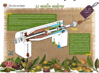
Fruits are ground by adjustable gap blades and paste is kneaded and then put in a powerful centrifuge that directly separates grignons\* from oil and water.
